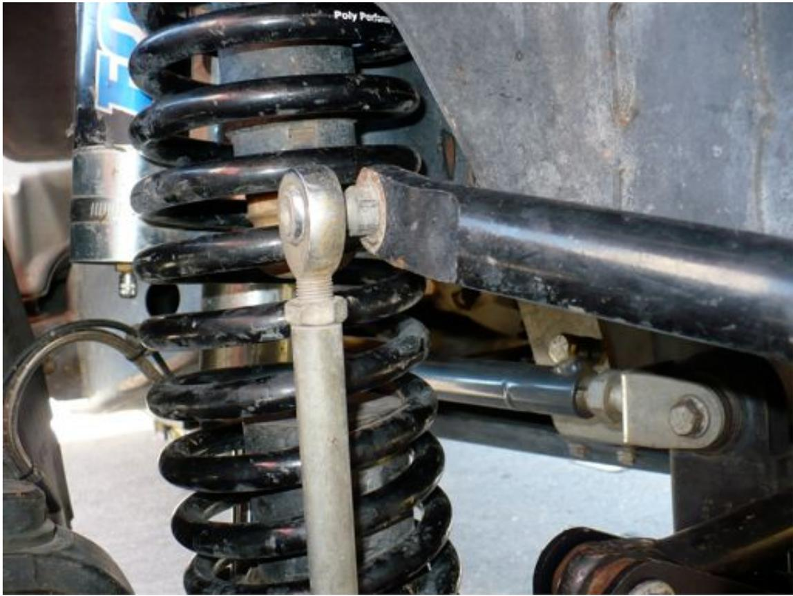
7. Attach the disconnect pins to the frame brackets using a flat washer on both sides and nylock nut as shown below. Slide the pins to the middle of the slotted hole. Tighten the nut to 40 ft-lbs.
