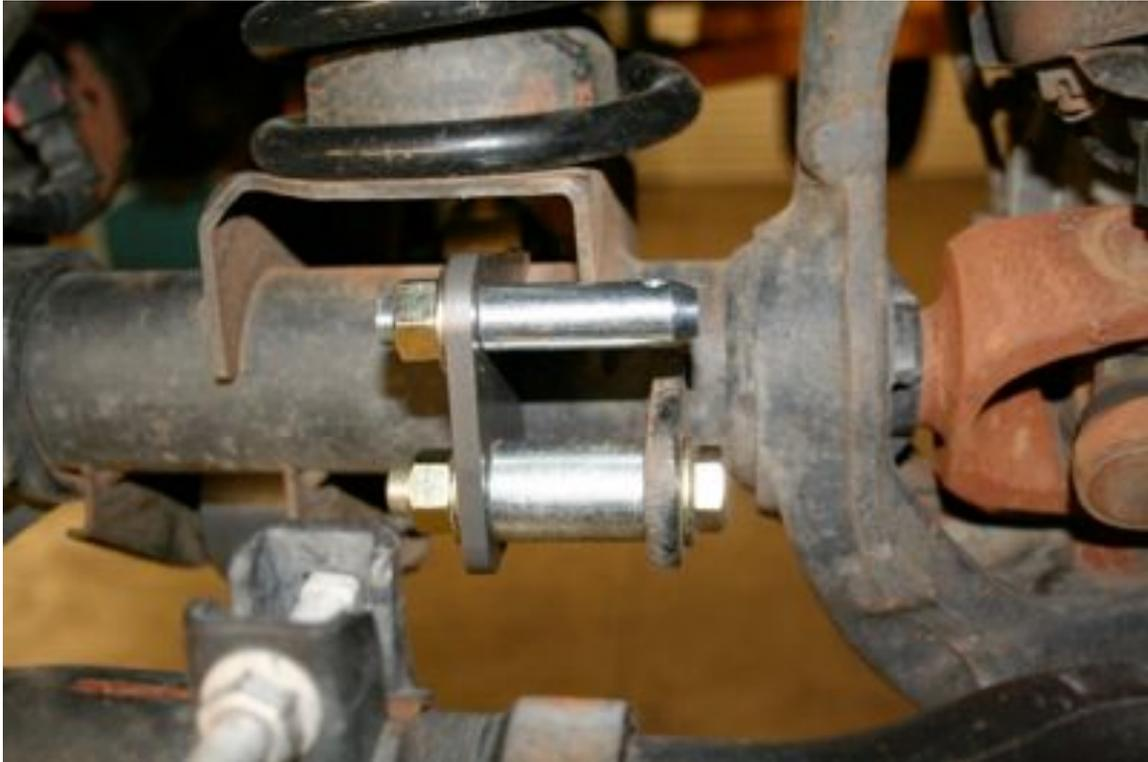
5. Adjust the sway bar links so both sides are the same length. Leave less than  $\frac{1}{2}$ " of thread showing past the jam nut. Tighten the jam nut so that the rod end stud is parallel to the lower bushing tube.
