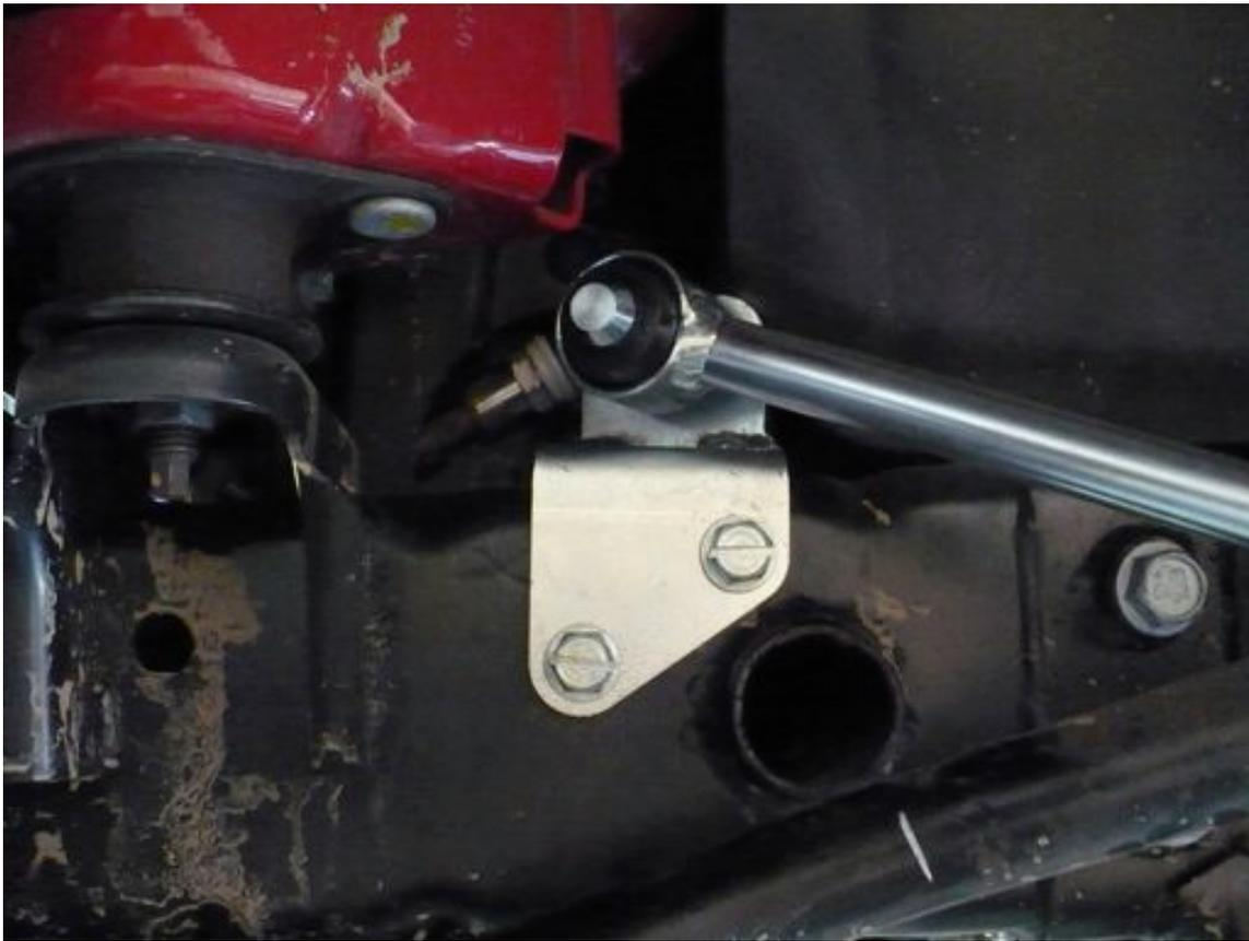
10. You can adjust the pins front to back in the frame bracket to allow easy attachment of the sway bar link.
