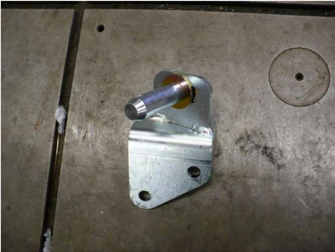
8. Position the sway bar end link mounting plates as shown below and slide the sway bar end link bushings onto the disconnect pin.
