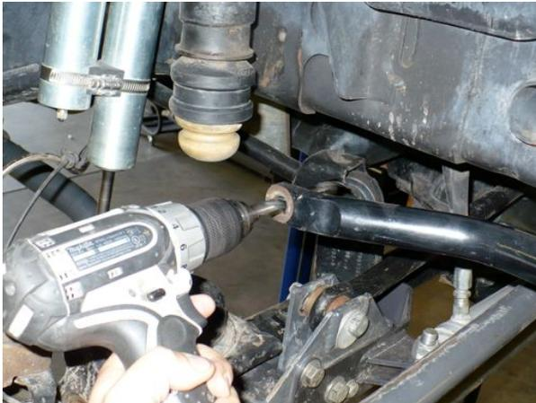
3. Attach the sway bar end link relocation brackets to the factory sway bar end link tab on the axle using the 1.5" long spacer and  $\frac{1}{2}$ " x 3" bolt. Use a flat washer under the bolt head and lock nut. The picture below shows the driver side relocation bracket; assemble the passenger side opposite of this.
