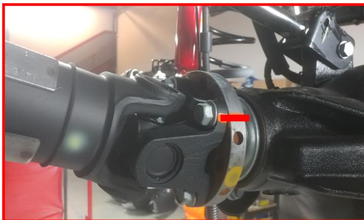
Remove the front drive shaft from differential.
