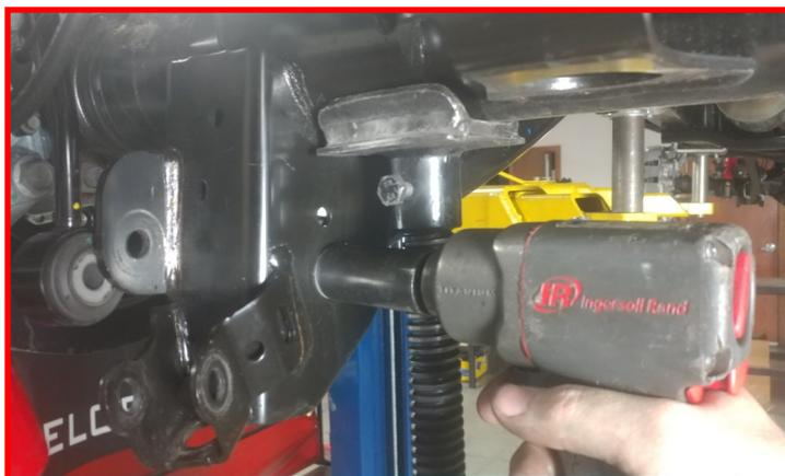
Loosen but do not remove the rear track bar at the axle and frame.
