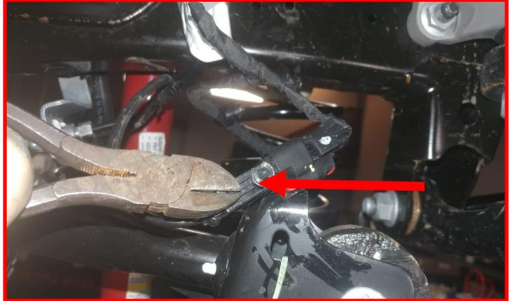
Remove the sway bar end links from the axle. Save the hardware.
