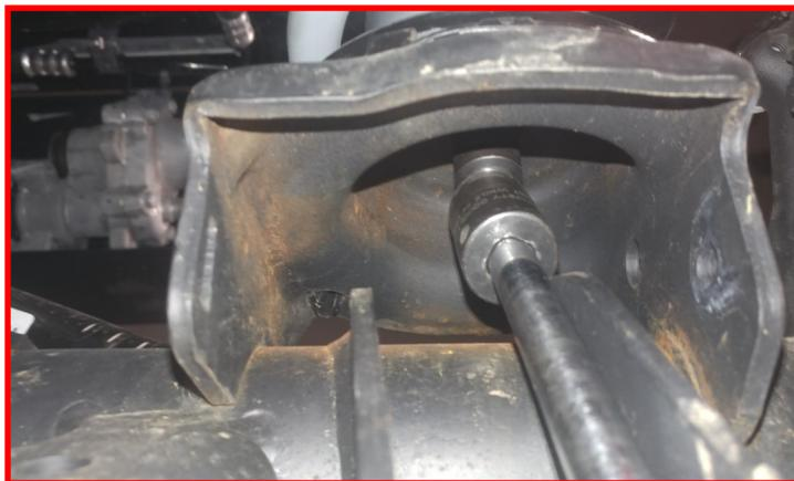
Locate the lower shock mounts on the axle and using a **1/2" drill bit**, drill out the hole in the bottom of the mount.
