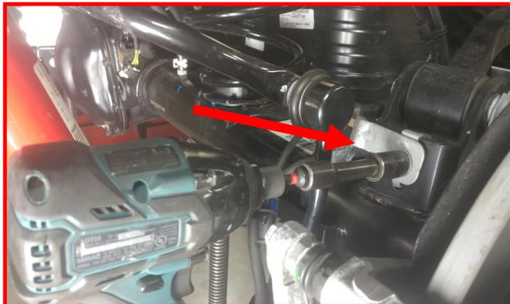
Remove the rear lower shock from the axle.
