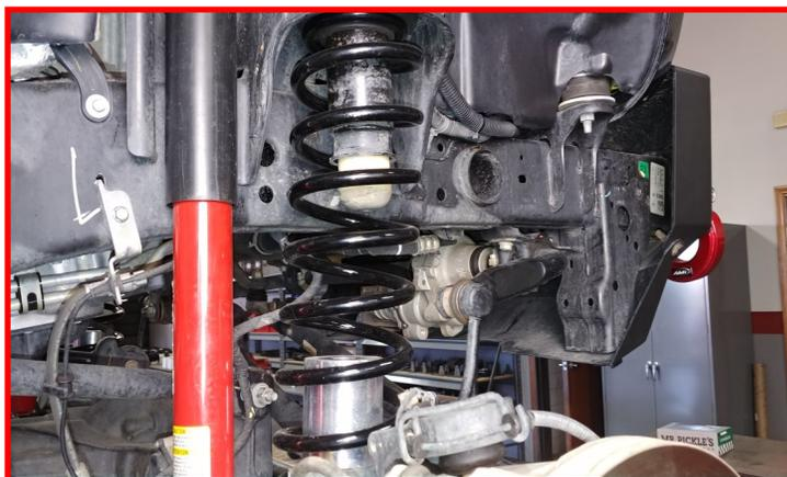
Remove the brake line bracket on the axle for access to install the bump stop nut on the passenger side for access to install the bump stop.
