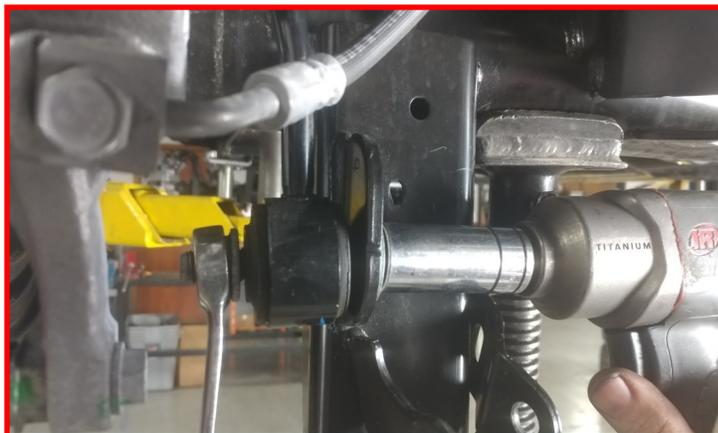
Remove the rear upper sway bar end link from the sway bar.
