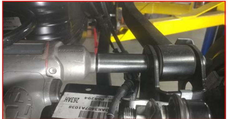
Loosen but do not remove the rear lower control arms at the axle and frame.
