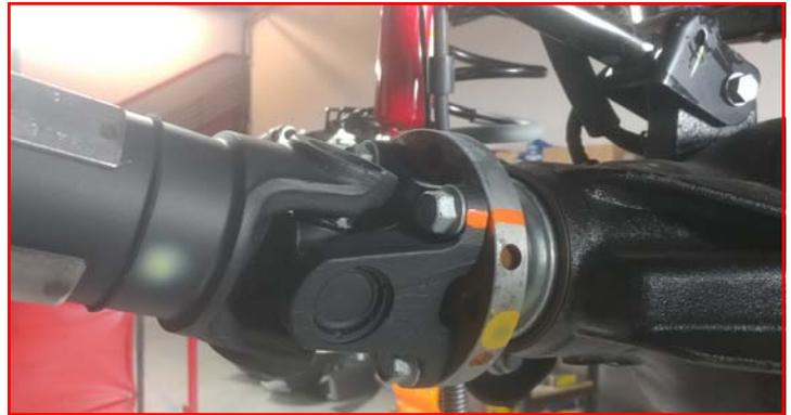
Remove the drive shaft from differential.
