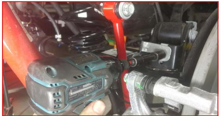
Install the ReadyLIFT rear bump stops to the axle using the provided **1/4" x .75" bolts, washers, and nuts**. Torque to **5 ft-lbs**.
