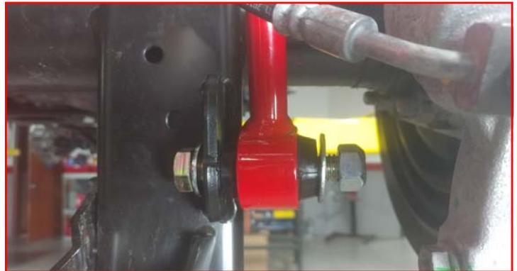
Install the ReadyLIFT rear shock extension using provided **1/2" x 1.25" bolt, washers, and nut.** Use the factory bolt to line up the holes while tightening the 1/2" hardware. Once tight, remove the factory hardware.
