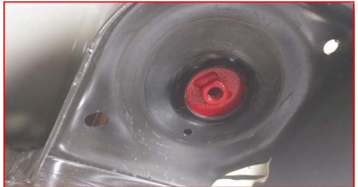
Install the ReadyLIFT rear spring spacer using the provided 1/2" x 2.25" Allen bolt. Torque to 25 ft-lbs.
