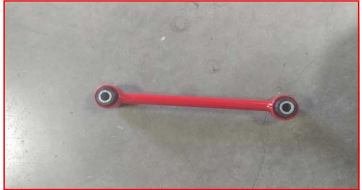
Install the ReadyLIFT sway bar end link to the sway bar using the factory lower hardware. Make sure to have the washer to the outside of the end link. Do not tighten at this time.
