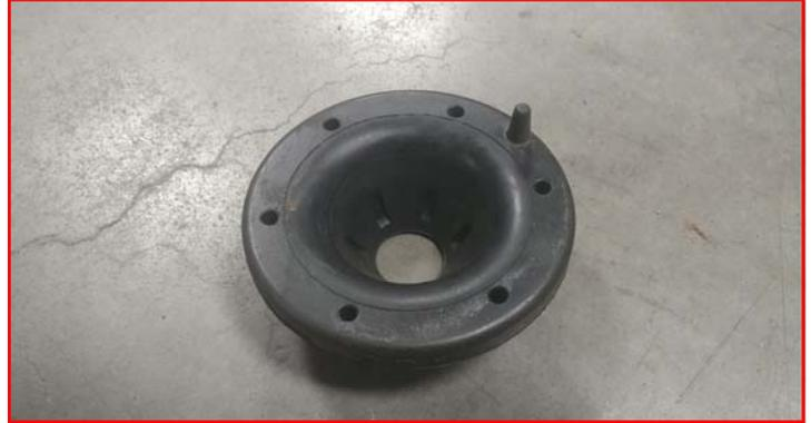
Remove the nipple off the rubber isolators using a suitable cutting device.
