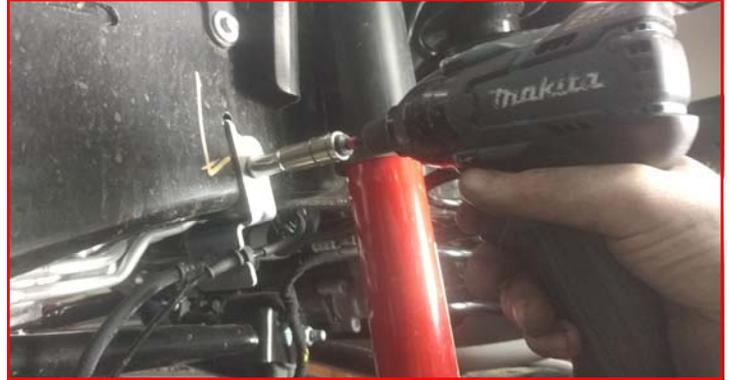
Remove the front brake line bracket at lower control arm.
