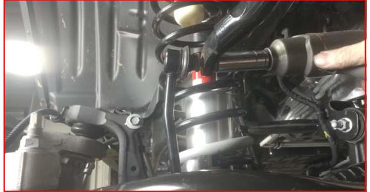
Install the front drive shaft making sure to line up the previous marks. Use a drop of thread locker on the factory hardware. Torque to **40 ft-lbs**.
