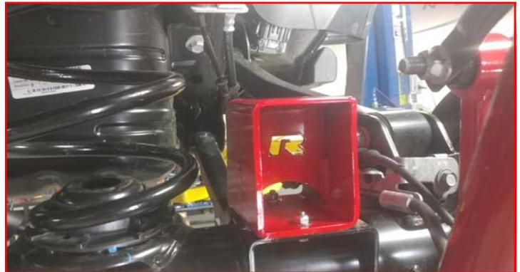
Install the wheels and lower the vehicle to the ground. Torque the lug nuts to the wheel manufacturer specs. Jounce the vehicle a few times to settle the suspension to the new ride height. Torque the upper control arms to **110 ft-lbs**, lower control arms and track bar hardware to **135 ft-lbs**, and shock and sway bar end link hardware to **50 ft-lbs**.
