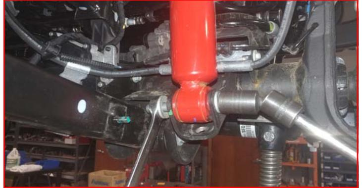
Loosen but do not remove the front lower control arms at the axle and frame.
