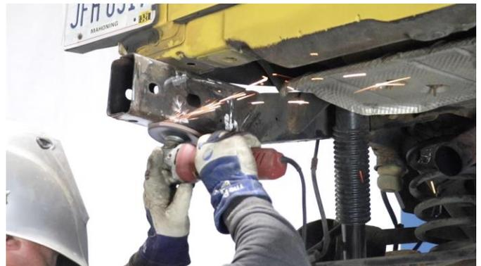
Hold the part up to the frame by roughly lining up the hole locations. Mark your intended cut line, removing as much rust as possible, while retaining a safe and weld-able margin.
