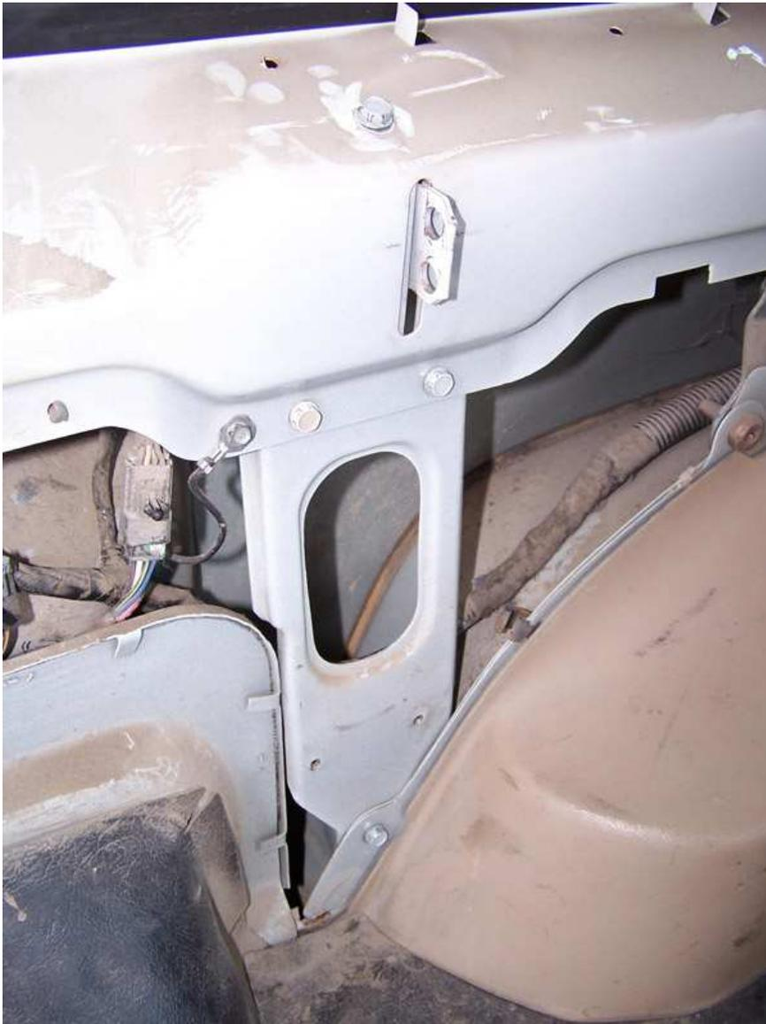
Now, hold up the LQG to the Jeep good and tight and mark the upper center hole. Set the LQG down and drill a 5/16" hole. Apply a small bead of RTV or silicon to the back of the guard being sure to make it around each bolt hole and the perimeter of the guard. Mount the LQG using the hole you just drilled. This will be enough to hold the weight of the LQG while you drill the rest of the holes.
