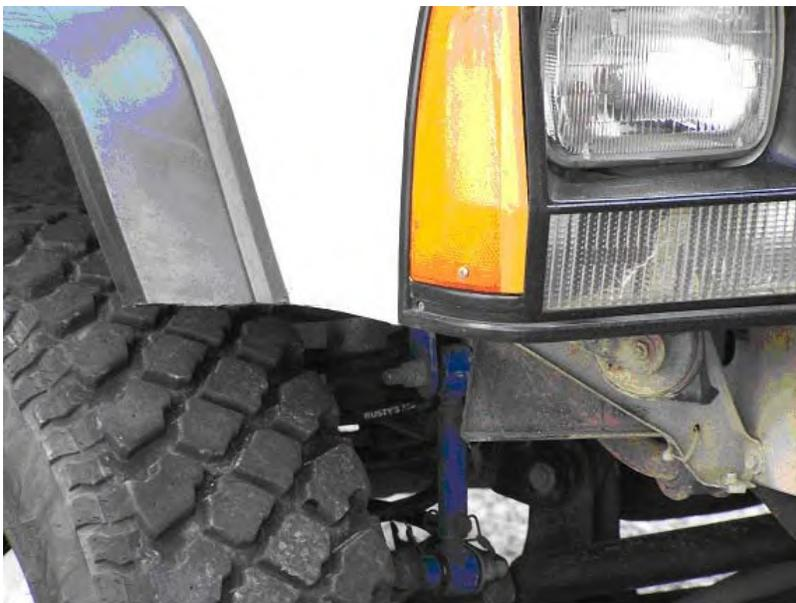
**Time to cut the fenders: (only 96 and earlier require fender trimming.)** I used a pneumatic cut off wheel. I made a straight cut starting at the headlight bezel and extending straight back to the fender flare. You can use whatever your preference is to cut sheet metal. It's best to use masking tape over the area to be cut to protect the finish and as a clean surface to mark the line.
