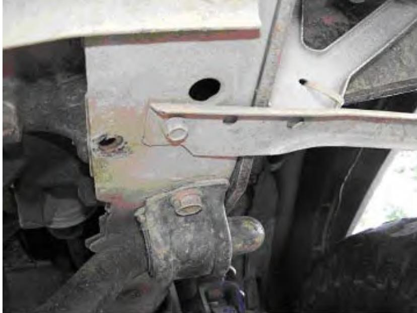
**Vacuum Canister:** On the passenger side of the jeep, mounted behind the bumper, is a vacuum canister. This canister will need to be removed for installation and re-installed. You can either use zip ties to fasten this to the fender brace or you can relocate it up into the engine compartment (ideal.)
