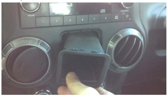
3. Remove the single 7mm bolt behind the switch panel.
