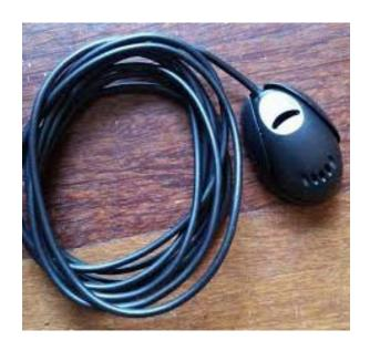
This external mic will work at just about any location, but we do have some recommendations as to placement. Try to keep this mic away from any windows, air vents, or speakers to avoid background sounds or feedback. The external mic will plug into the back of the JK1001 via a 3.5mm headphone jack plug located just to the left of the RCA pigtail.
