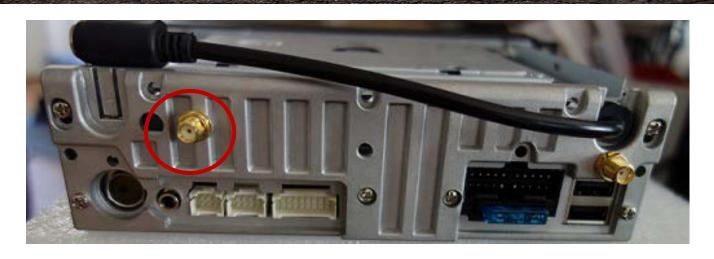
Above is a picture of the back of your JK1001. If your JK1001 is equipped with a Wi-Fi antenna, then you will have this additional gold plated plug just above the RCA plug in.
