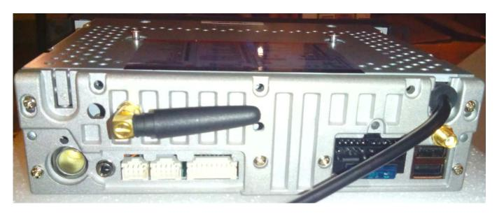
Your Wi-Fi antenna will screw on as shown above. Along with that, your GPS plug in is now on the far right hand side of the JK1001.
