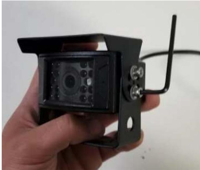
**Run the 4-pin camera harness to the location of the monitor and connect to the 4-pin connector on the monitor. Turn the monitor on and the image will be displayed. If not change the video input.**
