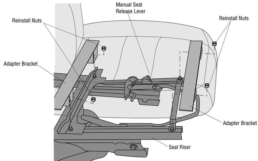
Note: In order to tumble the seat forward to access the rear of the vehicle, reach under the seat and manually push down on the Seat Release Lever.
