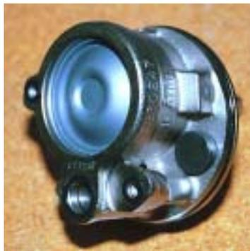
Inspect the new pump to make certain it is the proper one for your application. Although all P-type pumps look very similar, there are distinct differences. All 1980 and newer vehicles with Saginaw pumps were equipped with metric thread pumps with an o-ring type pressure fitting. 1979 and earlier vehicles were equipped with SAE thread pumps using a flare type fitting.
