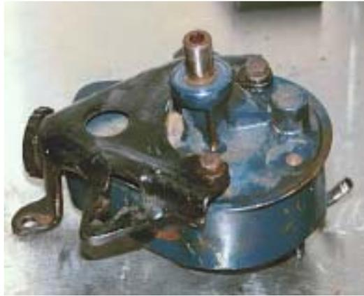
**Step 3** Remove the bolts or stud bolts from the back of the pump. In most applications there are two, but some only have one.
