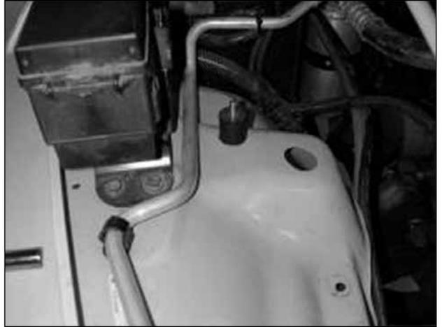
c. Install the supplied 6mm rubber mount. Use the supplied 6mm nut and 6mm washer. Attach the bolt and secure from underneath the fender well.
