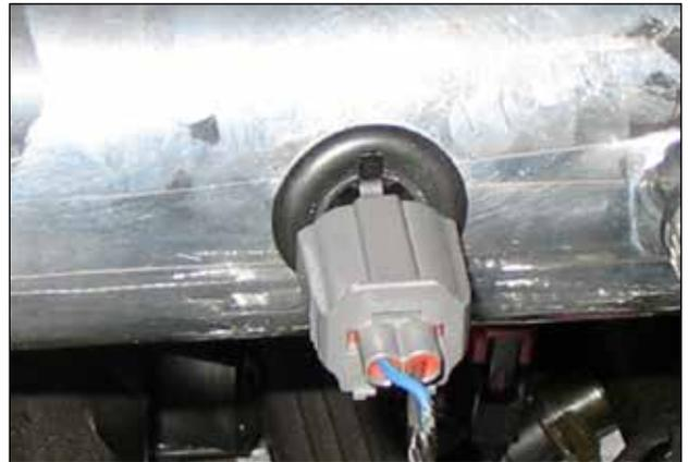
i. 2005-2006 Vehicles: Carefully install the IAT sensor into the intake pipe.
