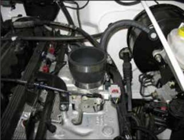
b. Secure the reducing coupler to the throttle body using the supplied #44 and #48 hose clamps.
