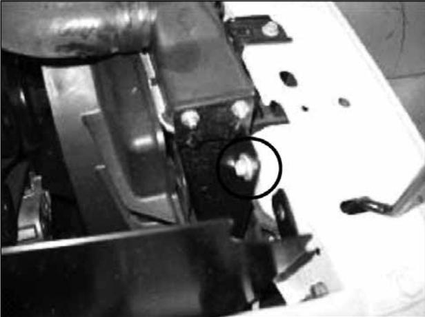
d. Remove the bolt securing the radiator to the core support. Slide the heat shield into position and re-insert the stock bolt through the heat shield hole and back through through the radiator support from which it was removed from.
