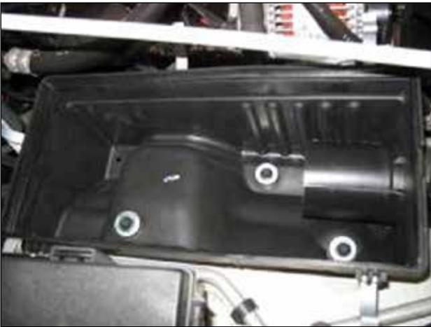
g. Remove the three bolts securing the bottom half of the air box to the vehicle.
