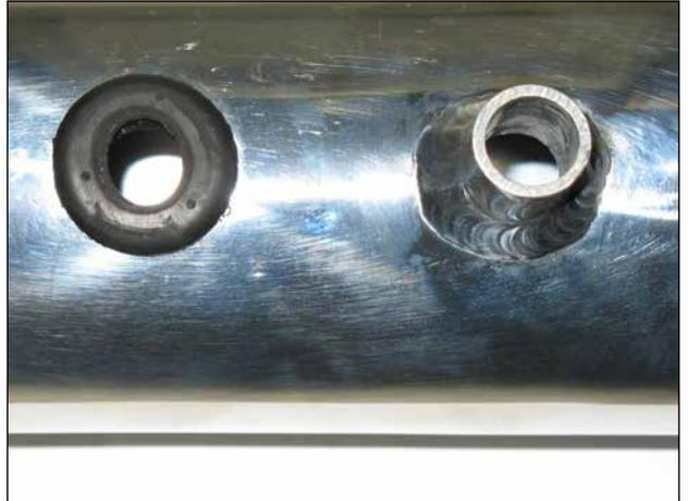
e. 2005-2006 Vehicles: Install the rubber grommet into the intake pipe as shown.
