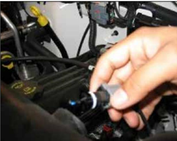
c. 2005-2006 Vehicles: Push in and twist the "Inlet Air Temperature" sensor out of the intake tube.
